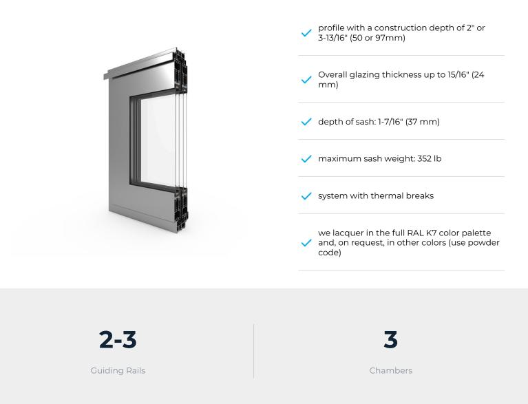
A system that ensures basic thermal insulation. Designed to produce sliding doors and windows that can be built into brick walls or as a part of aluminum facades or shopwindows made of elements of the MB-59 system.
