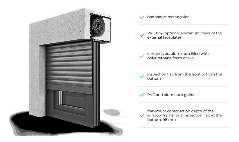
The system is unique for the best parameters of thermal and acoustic insulation due to its unique structure and very high quality of the components used. It allows you to provide comfort to users both in summer and winter. Thanks to the grooved front plates, there is no need to use additional plaster carriers when mounted on the outside and inside.
