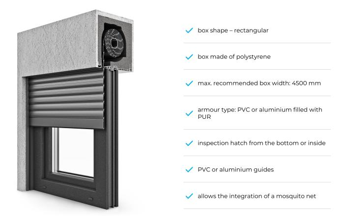
The Exte Neo XT top-mounted roller shutter is the so-called polystyrene system, which means that it is characterized by good parameters in terms of acoustic and thermal insulation. It is available in two revision versions – with a hatch from the bottom or from the inside – and with 9 different variants of boxes for the investor's convenience.
